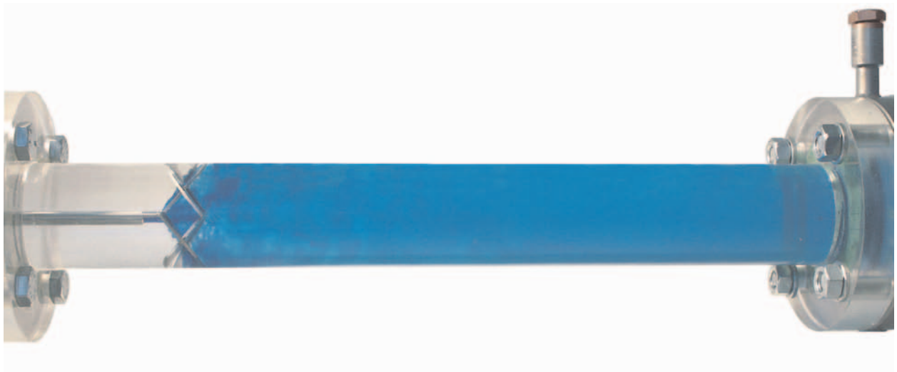
Fig. 1 5% of blue additive is dosed direct before an Aquamix/Flash Mixer ( Re = 18'000 )
