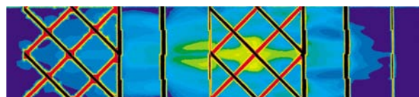
Fig. 5: CFD calculations of the CSE-X® mixer
