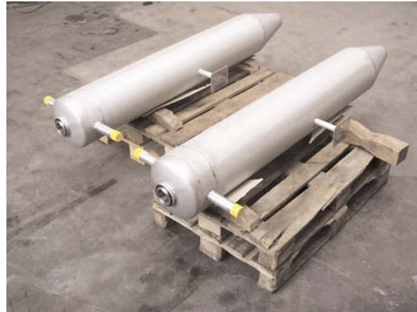
Fig. 5: CSE-XR® Polymer cooler for PET-melts
